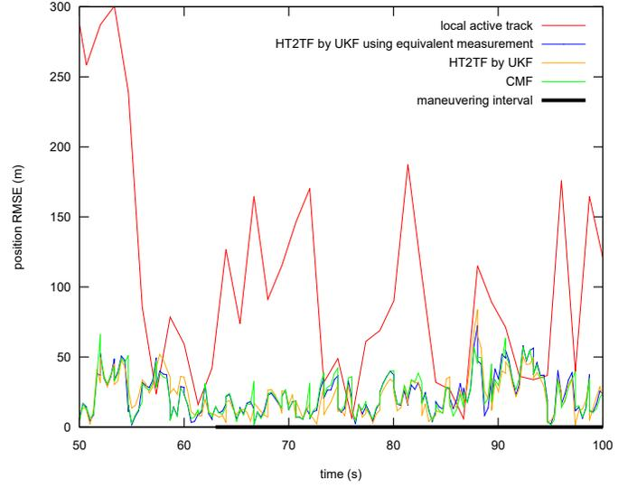
Fig. 2. RMSE for the position for  $50 \text{ s} < t < 100 \text{ s}$  of the global tracker, the local active tracker and the two references.
