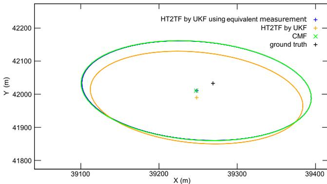
Fig. 4. Position estimation and its associated uncertainty of the global tracker and the two references. The ground truth is displayed additionally.
